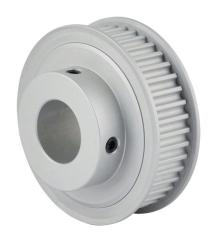
Sung-Il Machinery timing pulley, aluminum, 5mm 5M pitch, 42 tooth, 2.632in pitch diameter, 7/8in bore, hub with flanges. For use with 15mm wide belt.
