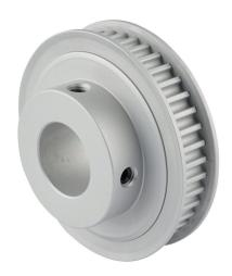
Sung-Il Machinery timing pulley, aluminum, 5mm 5M pitch, 42 tooth, 2.632in pitch diameter, 7/8in bore, hub with flanges. For use with 9mm wide belt.
