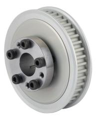
Sung-Il Machinery timing pulley, aluminum, 5mm 5M pitch, 42 tooth, 2.632in pitch diameter, 5/8in bore, no hub with flanges. For use with 9mm wide belt. QD bushing included.
