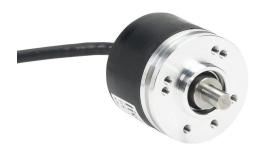
Lika Electronic A41 series incremental (quadrature) rotary encoder, light duty, 5-30 VDC, axial exit, universal (line driver or NPN/PNP open collector) output, 4096 ppr, 1/4in solid shaft, 41mm diameter body, IP64, 6.5ft/2m cable length, pigtail.
