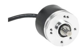
Lika Electronic A41 series incremental (quadrature) rotary encoder, light duty, 5-30 VDC, axial exit, universal (line driver or NPN/PNP open collector) output, 3600 ppr, 1/4in solid shaft, 41mm diameter body, IP64, 6.5ft/2m cable length, pigtail.
