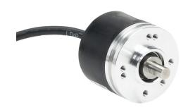
Lika Electronic A41 series incremental (quadrature) rotary encoder, light duty, 5-30 VDC, axial exit, universal (line driver or NPN/PNP open collector) output, 2048 ppr, 1/4in solid shaft, 41mm diameter body, IP64, 6.5ft/2m cable length, pigtail.
