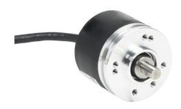
Lika Electronic A41 series incremental (quadrature) rotary encoder, light duty, 5-30 VDC, axial exit, universal (line driver or NPN/PNP open collector) output, 2000 ppr, 1/4in solid shaft, 41mm diameter body, IP64, 6.5ft/2m cable length, pigtail.
