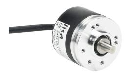
Lika Electronic A41 series incremental (quadrature) rotary encoder, light duty, 5-30 VDC, axial exit, universal (line driver or NPN/PNP open collector) output, 1024 ppr, 1/4in solid shaft, 41mm diameter body, IP64, 6.5ft/2m cable length, pigtail.
