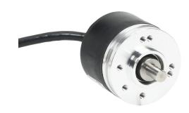
Lika Electronic A41 series incremental (quadrature) rotary encoder, light duty, 5-30 VDC, axial exit, universal (line driver or NPN/PNP open collector) output, 1000 ppr, 1/4in solid shaft, 41mm diameter body, IP64, 6.5ft/2m cable length, pigtail.
