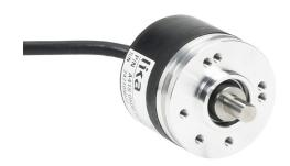
Lika Electronic A41 series incremental (quadrature) rotary encoder, light duty, 5-30 VDC, axial exit, universal (line driver or NPN/PNP open collector) output, 500 ppr, 1/4in solid shaft, 41mm diameter body, IP64, 6.5ft/2m cable length, pigtail.
