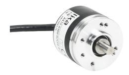
Lika Electronic A41 series incremental (quadrature) rotary encoder, light duty, 5-30 VDC, axial exit, universal (line driver or NPN/PNP open collector) output, 360 ppr, 1/4in solid shaft, 41mm diameter body, IP64, 6.5ft/2m cable length, pigtail.
