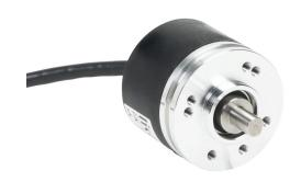
Lika Electronic A41 series incremental (quadrature) rotary encoder, light duty, 5-30 VDC, axial exit, universal (line driver or NPN/PNP open collector) output, 200 ppr, 1/4in solid shaft, 41mm diameter body, IP64, 6.5ft/2m cable length, pigtail.
