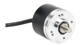
Lika Electronic A41 series incremental (quadrature) rotary encoder, light duty, 5-30 VDC, axial exit, universal (line driver or NPN/PNP open collector) output, 100 ppr, 1/4in solid shaft, 41mm diameter body, IP64, 6.5ft/2m cable length, pigtail.
