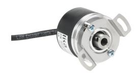
Lika Electronic A41 series incremental (quadrature) rotary encoder, light duty, 5-30 VDC, axial exit, universal (line driver or NPN/PNP open collector) output, 4096 ppr, 1/4in hollow shaft, 41mm diameter body, IP64, 6.5ft/2m cable length, pigtail.
