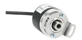
Lika Electronic A41 series incremental (quadrature) rotary encoder, light duty, 5-30 VDC, axial exit, universal (line driver or NPN/PNP open collector) output, 3600 ppr, 1/4in hollow shaft, 41mm diameter body, IP64, 6.5ft/2m cable length, pigtail.
