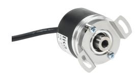
Lika Electronic A41 series incremental (quadrature) rotary encoder, light duty, 5-30 VDC, axial exit, universal (line driver or NPN/PNP open collector) output, 2048 ppr, 1/4in hollow shaft, 41mm diameter body, IP64, 6.5ft/2m cable length, pigtail.
