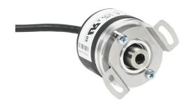
Lika Electronic A41 series incremental (quadrature) rotary encoder, light duty, 5-30 VDC, axial exit, universal (line driver or NPN/PNP open collector) output, 2000 ppr, 1/4in hollow shaft, 41mm diameter body, IP64, 6.5ft/2m cable length, pigtail.
