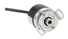
Lika Electronic A41 series incremental (quadrature) rotary encoder, light duty, 5-30 VDC, axial exit, universal (line driver or NPN/PNP open collector) output, 1024 ppr, 1/4in hollow shaft, 41mm diameter body, IP64, 6.5ft/2m cable length, pigtail.
