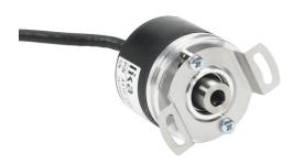
Lika Electronic A41 series incremental (quadrature) rotary encoder, light duty, 5-30 VDC, axial exit, universal (line driver or NPN/PNP open collector) output, 1000 ppr, 1/4in hollow shaft, 41mm diameter body, IP64, 6.5ft/2m cable length, pigtail.
