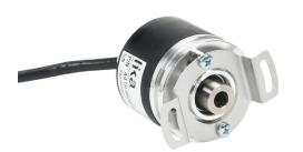
Lika Electronic A41 series incremental (quadrature) rotary encoder, light duty, 5-30 VDC, axial exit, universal (line driver or NPN/PNP open collector) output, 500 ppr, 1/4in hollow shaft, 41mm diameter body, IP64, 6.5ft/2m cable length, pigtail.
