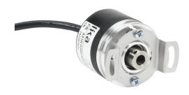
Lika Electronic A41 series incremental (quadrature) rotary encoder, light duty, 5-30 VDC, axial exit, universal (line driver or NPN/PNP open collector) output, 360 ppr, 1/4in hollow shaft, 41mm diameter body, IP64, 6.5ft/2m cable length, pigtail.
