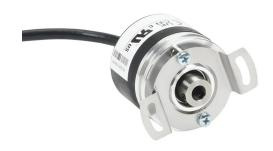
Lika Electronic A41 series incremental (quadrature) rotary encoder, light duty, 5-30 VDC, axial exit, universal (line driver or NPN/PNP open collector) output, 200 ppr, 1/4in hollow shaft, 41mm diameter body, IP64, 6.5ft/2m cable length, pigtail.
