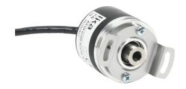
Lika Electronic A41 series incremental (quadrature) rotary encoder, light duty, 5-30 VDC, axial exit, universal (line driver or NPN/PNP open collector) output, 100 ppr, 1/4in hollow shaft, 41mm diameter body, IP64, 6.5ft/2m cable length, pigtail.
