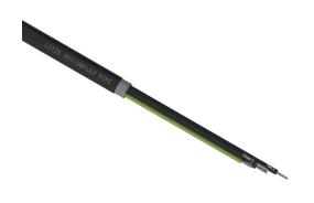
LUTZE MOTIONFLEX continuous flexing VFD cable, shielded, 4 conductors (includes ground), 18 AWG, 41-stranded, tinned copper, XLPE conductor insulation material, XHHW-2 jacket, black, cut to length.
