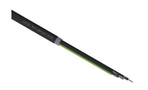
LUTZE MOTIONFLEX continuous flexing VFD cable, shielded, 4 conductors (includes ground), 16 AWG, 65-stranded, tinned copper, XLPE conductor insulation material, XHHW-2 jacket, black, cut to length.
