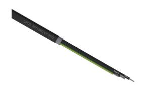
LUTZE MOTIONFLEX continuous flexing VFD cable, shielded, 4 conductors (includes ground), 14 AWG, 104-stranded, tinned copper, XLPE conductor insulation material, XHHW-2 jacket, black, cut to length.
