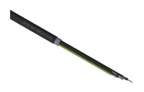
LUTZE MOTIONFLEX continuous flexing VFD cable, shielded, 4 conductors (includes ground), 12 AWG, 168-stranded, tinned copper, XLPE conductor insulation material, XHHW-2 jacket, black, cut to length.
