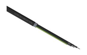
LUTZE MOTIONFLEX continuous flexing VFD cable, shielded, 4 conductors (includes ground), 10 AWG, 259-stranded, tinned copper, XLPE conductor insulation material, XHHW-2 jacket, black, cut to length.
