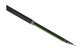
LUTZE MOTIONFLEX continuous flexing VFD cable, shielded, 4 conductors (includes ground), 8 AWG, 336-stranded, tinned copper, XLPE conductor insulation material, XHHW-2 jacket, black, cut to length.
