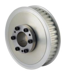
Sung-II Machinery timing pulley, aluminum, 3/8in L pitch, 40 tooth, 4.775in pitch diameter, 1-1/4in bore, no hub with flanges. For use with 1in wide belt. QD bushing included.
