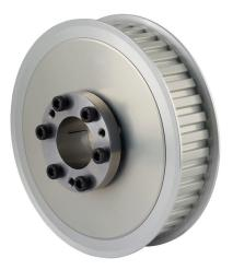
Sung-Il Machinery timing pulley, aluminum, 3/8in L pitch, 40 tooth, 4.775in pitch diameter, 1-1/8in bore, no hub with flanges. For use with 1in wide belt. QD bushing included.
