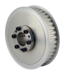
Sung-II Machinery timing pulley, aluminum, 3/8in L pitch, 40 tooth, 4.775in pitch diameter, 1-1/8in bore, no hub with flanges. For use with 1in wide belt. QD bushing included.
