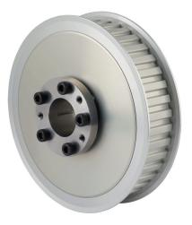
Sung-Il Machinery timing pulley, aluminum, 3/8in L pitch, 40 tooth, 4.775in pitch diameter, 1in bore, no hub with flanges. For use with 1in wide belt. QD bushing included.
