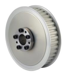
Sung-Il Machinery timing pulley, aluminum, 3/8in L pitch, 40 tooth, 4.775in pitch diameter, 7/8in bore, no hub with flanges. For use with 1in wide belt. QD bushing included.
