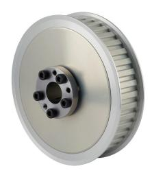
Sung-Il Machinery timing pulley, aluminum, 3/8in L pitch, 40 tooth, 4.775in pitch diameter, 3/4in bore, no hub with flanges. For use with 1in wide belt. QD bushing included.
