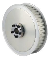
Sung-Il Machinery timing pulley, aluminum, 3/8in L pitch, 40 tooth, 4.775in pitch diameter, 5/8in bore, no hub with flanges. For use with 1in wide belt. QD bushing included.
