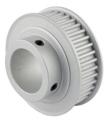
Sung-Il Machinery timing pulley, aluminum, 5mm 5M pitch, 40 tooth, 2.506in pitch diameter, 1-1/8in bore, hub with flanges. For use with 15mm wide belt.
