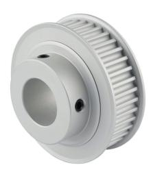
Sung-Il Machinery timing pulley, aluminum, 5mm 5M pitch, 40 tooth, 2.506in pitch diameter, 7/8in bore, hub with flanges. For use with 15mm wide belt.
