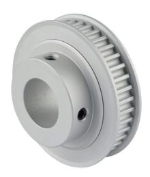
Sung-II Machinery timing pulley, aluminum, 5mm 5M pitch, 40 tooth, 2.506in pitch diameter, 7/8in bore, hub with flanges. For use with 9mm wide belt.
