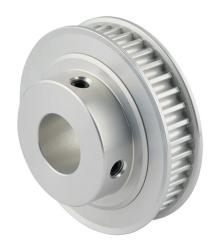
Sung-II Machinery timing pulley, aluminum, 5mm 5M pitch, 40 tooth, 2.506in pitch diameter, 3/4in bore, hub with flanges. For use with 9mm wide belt.
