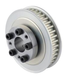
Sung-Il Machinery timing pulley, aluminum, 5mm 5M pitch, 40 tooth, 2.506in pitch diameter, 5/8in bore, no hub with flanges. For use with 9mm wide belt. QD bushing included.
