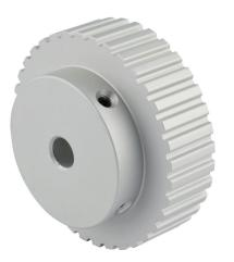
Sung-Il Machinery timing pulley, aluminum, 1/5in XL pitch, 36 tooth, 2.292in pitch diameter, 5/16in bore, hub without flanges. For use with 3/8in wide belt.
