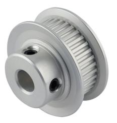
Sung-Il Machinery timing pulley, aluminum, 0.08in MXL pitch, 36 tooth, 0.917in pitch diameter, 1/4in bore, hub with flanges. For use with 1/4in wide belt.
