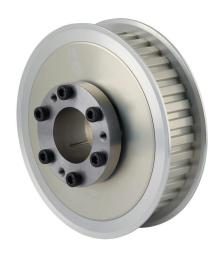
Sung-II Machinery timing pulley, aluminum, 3/8in L pitch, 36 tooth, 4.297in pitch diameter, 1-1/4in bore, no hub with flanges. For use with 1in wide belt. QD bushing included.
