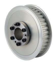
Sung-II Machinery timing pulley, aluminum, 3/8in L pitch, 36 tooth, 4.297in pitch diameter, 1-1/8in bore, no hub with flanges. For use with 1in wide belt. QD bushing included.
