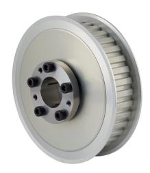
Sung-Il Machinery timing pulley, aluminum, 3/8in L pitch, 36 tooth, 4.297in pitch diameter, 1in bore, no hub with flanges. For use with 1in wide belt. QD bushing included.
