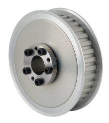
Sung-Il Machinery timing pulley, aluminum, 3/8in L pitch, 36 tooth, 4.297in pitch diameter, 7/8in bore, no hub with flanges. For use with 1in wide belt. QD bushing included.
