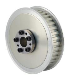
Sung-Il Machinery timing pulley, aluminum, 3/8in L pitch, 36 tooth, 4.297in pitch diameter, 3/4in bore, no hub with flanges. For use with 1in wide belt. QD bushing included.
