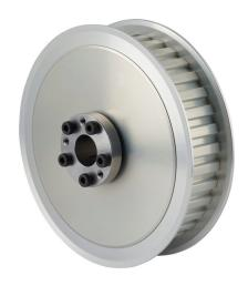
Sung-Il Machinery timing pulley, aluminum, 3/8in L pitch, 36 tooth, 4.297in pitch diameter, 5/8in bore, no hub with flanges. For use with 1in wide belt. QD bushing included.
