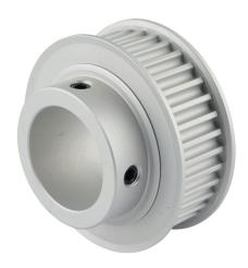
Sung-II Machinery timing pulley, aluminum, 5mm 5M pitch, 36 tooth, 2.256in pitch diameter, 1-1/8in bore, hub with flanges. For use with 15mm wide belt.
