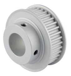
Sung-Il Machinery timing pulley, aluminum, 5mm 5M pitch, 36 tooth, 2.256in pitch diameter, 7/8in bore, hub with flanges. For use with 15mm wide belt.
